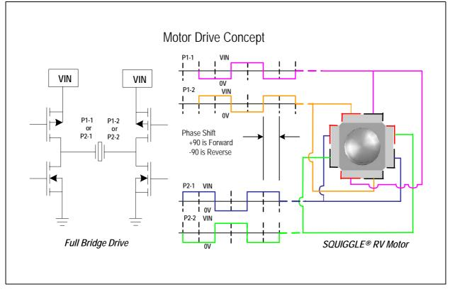
Figure 4. Motor Drive Concept (UTAF Motor)
